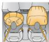
Front airbags supplement seat belts to help protect the head and chest of the driver and passenger in front.
