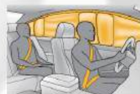
Side curtain airbags can help protect the heads of outboard occupants during a side impact.
