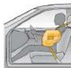
Side airbags can help reduce chest injuries to front-seat occupants during severe side impacts.
